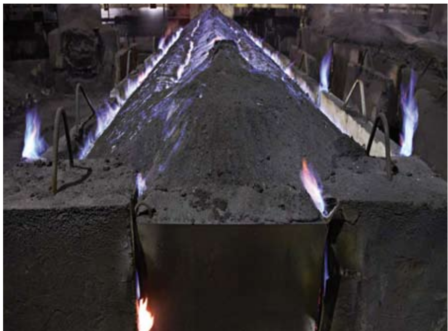
A carborex-grade SiC furnace operated by Washington Mills, on-line at more than 2,000°C. Courtesy Washington Mills AS
